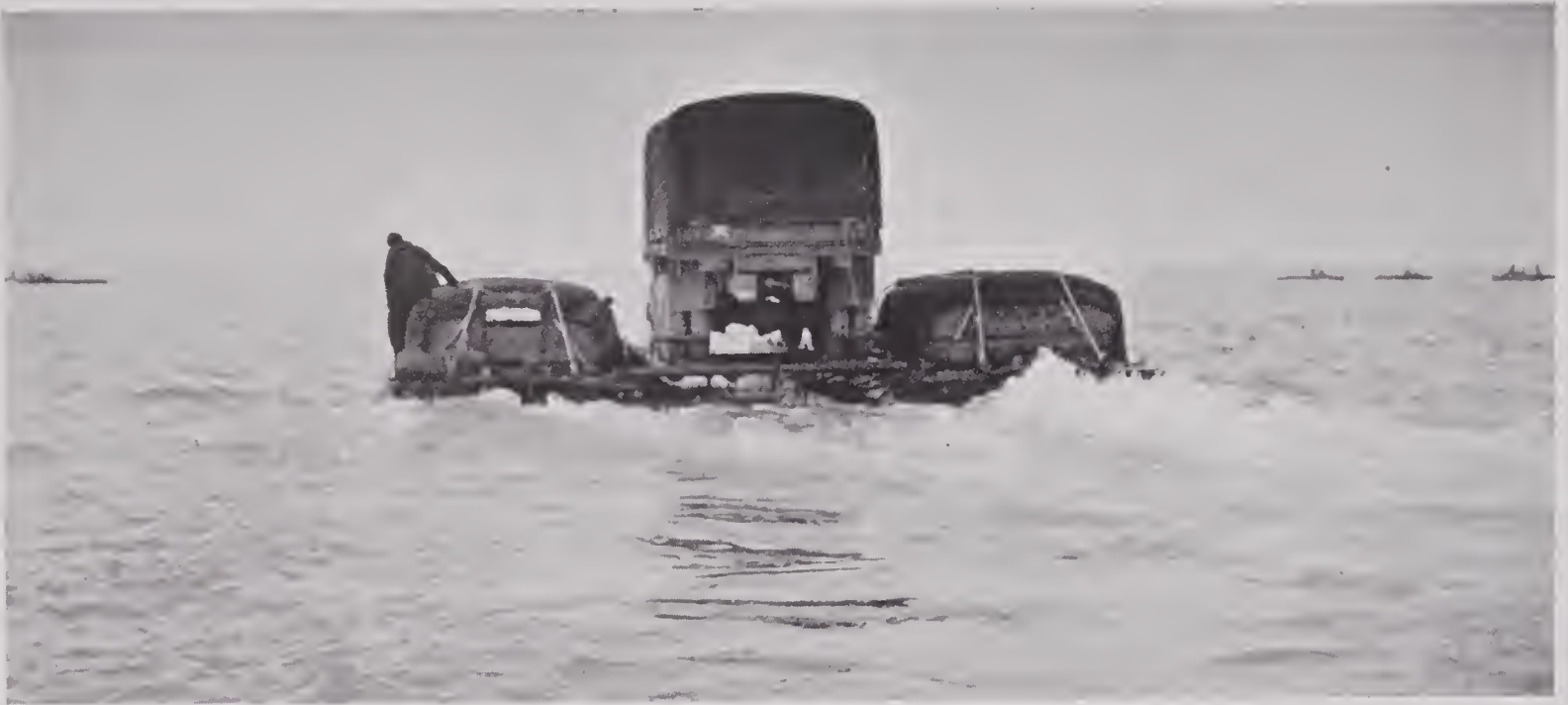
FIGURE 70. Truck at sea in test of DUKW dry ferry.
